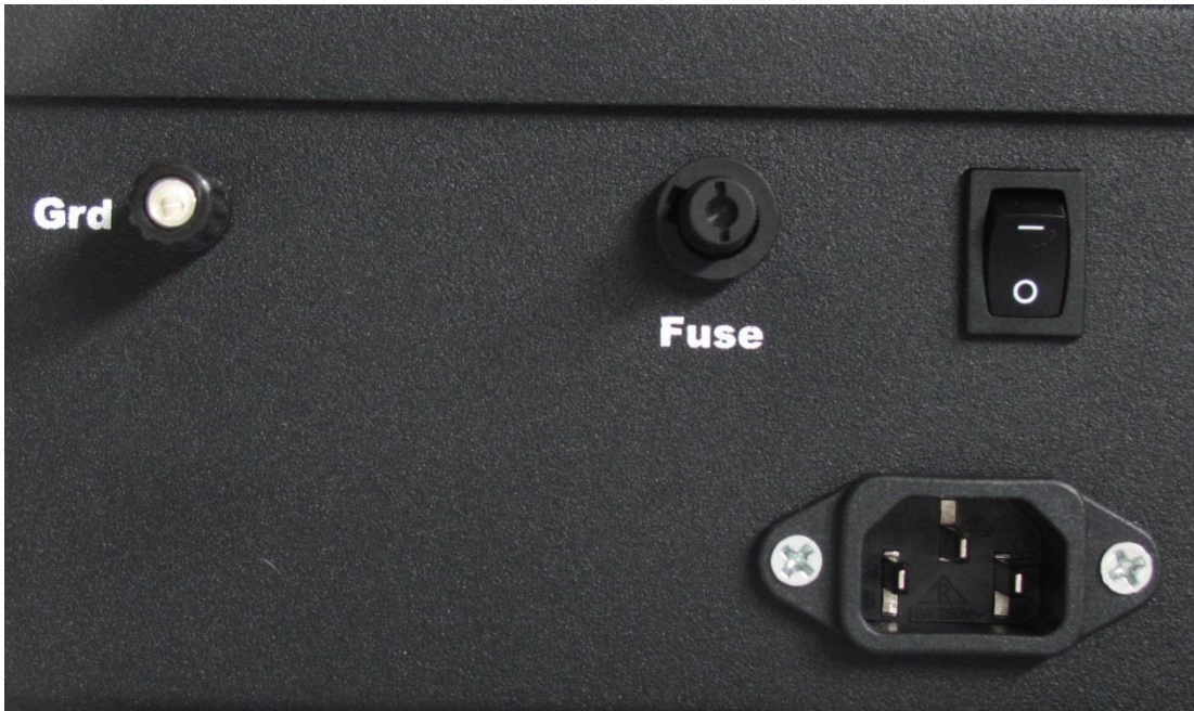
Figure 4A – End of PS box with socket for power cord.
