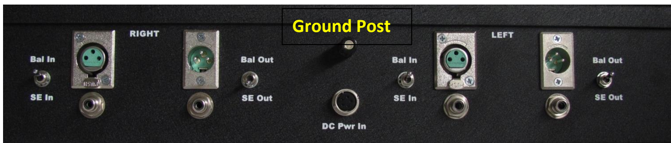
Figure 3 – Rear panel showing connectors.
